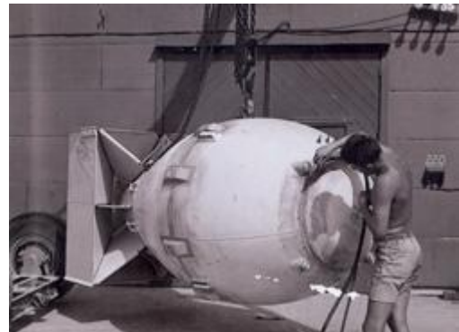
The polar cap of the "Fat Man" weapon being sprayed with plastic spray paint in front of Assembly Building Number 2. (Photo from U.S. National Archives, RG 77-BT)
