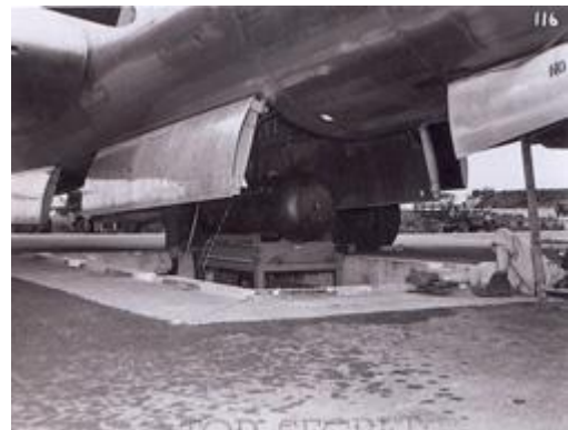
This shows "Little Boy" being raised for loading into the Enola Gay's bomb bay. (Photo from U.S. National Archives, RG 77-BT)
