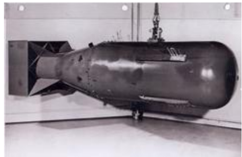
A nuclear weapon of the "Little Boy" type, the uranium gun-type detonated over Hiroshima. It is 28 inches in diameter and 120 inches long. "Little Boy" weighed about 9,000 pounds and had a yield approximating 15,000 tons of high explosives. (Copy from U.S. National Archives, RG 77-AEC)
